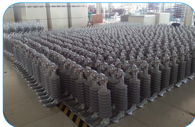
Composite line post insulators
