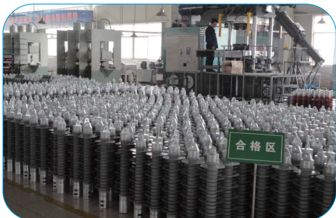
Composite railway insulators
